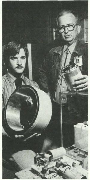
DRAMATIC DIFFERENCE in capacitor technology is demonstrated by Gary Webb, holding conventional capacitor, and Howie Mauldin (both 2316), holding newly developed capacitor with perfluorocarbon impregnating agent. Both capacitors have the same rated output.
